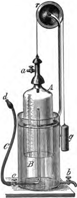
Fig. 247.—Wintrich's modification of Hutchinson's spirometer.—(Reichert.)
